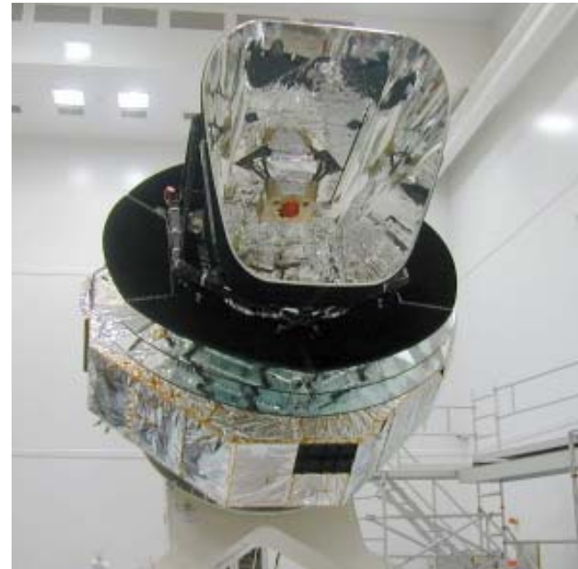
Planck Cryo Qualification Model under test at CSL, Liège.
